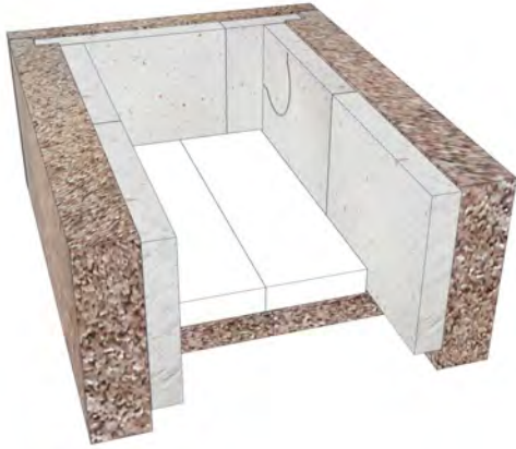
Abb. 2-1: Brennkammer (SH20, SH30)
