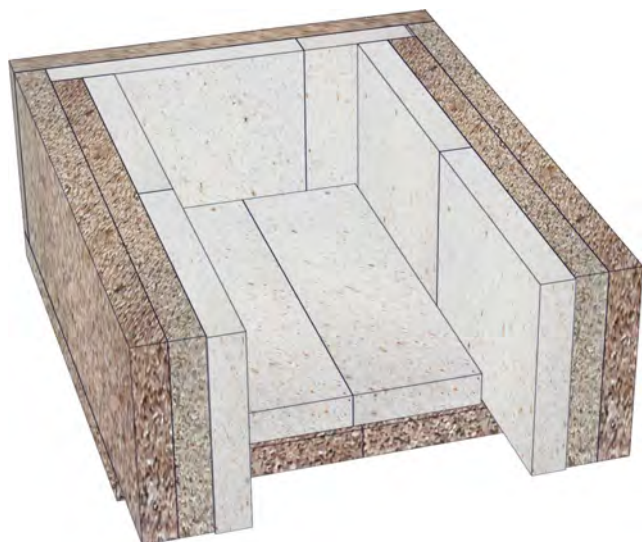
Abb. 2-1: Brennkammer (SH20, SH30)
