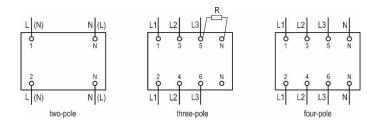
RCCB in a three-phase system without a neutral conductor: The N terminal should be connected to terminal 5 or 6 via the Rresistor, depending on the supply side, in order to keep 230 V power supply voltage of the test circuit. Test current is wrong if the value of the R resistor is incorrect or if only a wire connection is used instead. The R resistor value is:
