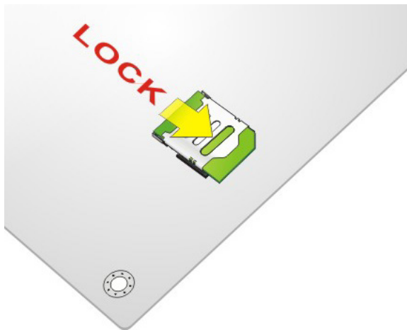
Figure 4-9: Lock SIM Card Slot Cover
