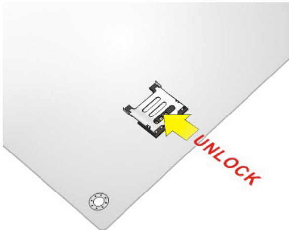
Figure 4-7: Unlock SIM Card Slot Cover
